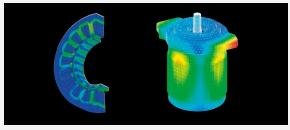
3D magnetic analysis of a direct drive (DD) motor (left) and magnetic vibration analysis of an EPS motor (right)
