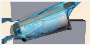
Computational fluid dynamics (CFD) analysis of tapered roller bearings
